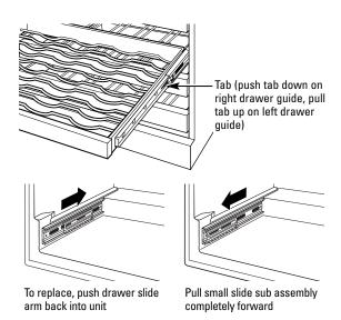
**NOTE:** Make sure the tabs on the full extension drawer guides are fully engaged before loading any bottles. Pull the drawers out all the way to the STOP position and push back in several times to make sure locking tabs are properly engaged.
